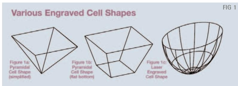
customary to chrome plate the roller for wear resistance. The individual cells manufactured by this process had a pyramid shape with either a pointed bottom or a truncated bottom. (Fig 1)
